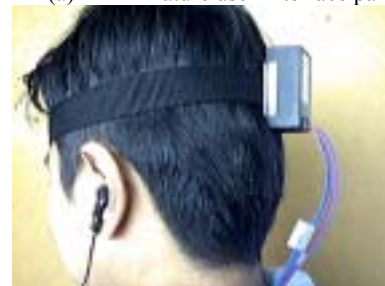
(b) Gyroscope sensor for head tracking
