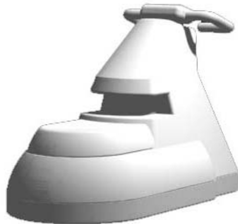
Fig. 10 Ergonomic design of the medical service mobile robot
