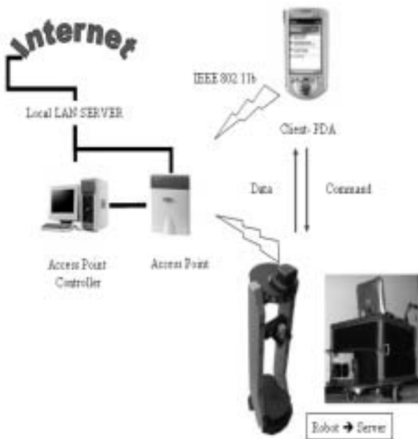
Fig. 9 Wireless communication application in the service mobile robot
