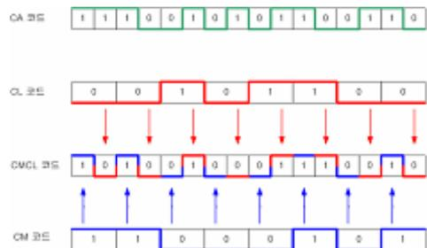
Fig 12. Mode Selector output codes.
