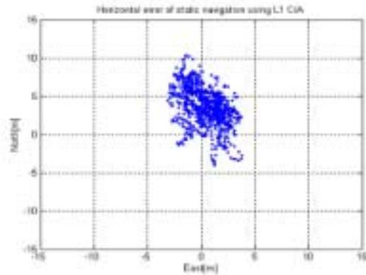
Fig 13. Horizontal error of static navigation (GPS L1 Signal).
