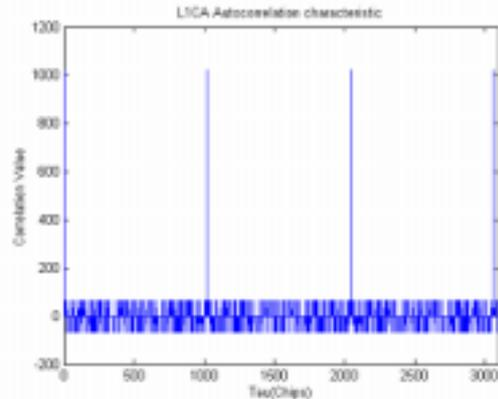
Fig 5. Autocorrelation characteristics of L1 C/A code
