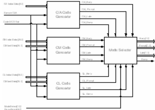
Fig 10. L1/L2CS Code Generator.
