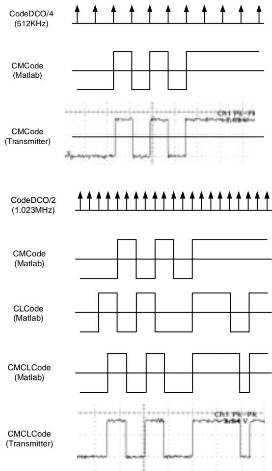
Fig 16. The output signals of Transmitter.
