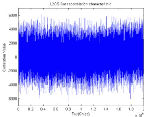
Fig 8. Cross correlation characteristics of L2CS code
