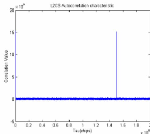
Fig 7. Autocorrelation characteristics of L2CS code
