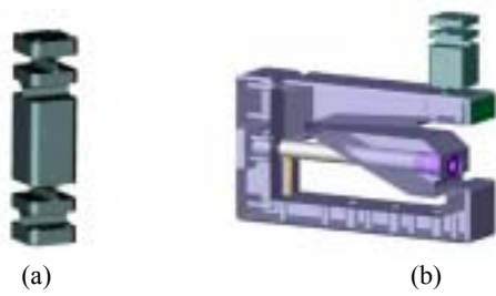
(a) Spherical joint with flexible structures (b) Double L type Amplification Hinge Module
