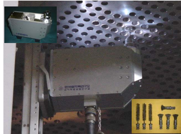
Fig. 12 Brushing tool and wire brushes.
