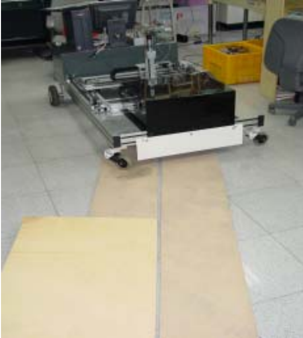
Fig.15 Crack tracking of mobile robot
