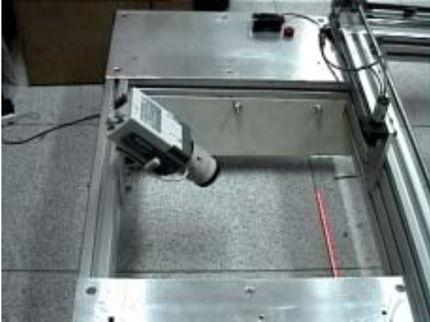
Fig.5 Crack detection device setup
