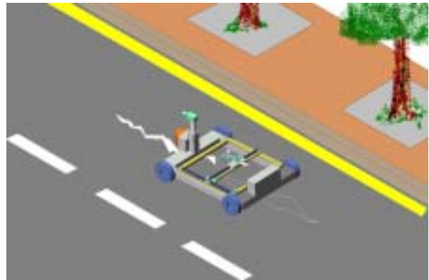
Fig.1 The crack sealing robot working environment.
