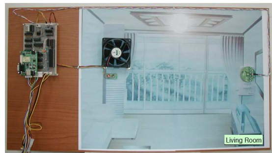
Fig. 8. Testbed for Heater A/C and temperature
