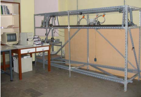
Fig. 5 Structure of overhead crane system.
