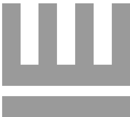
(c) Anisotropic etch using RIE
