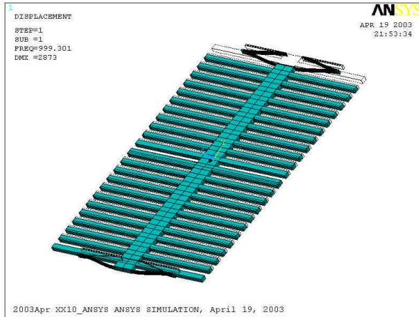
Figure 2 Modal analysis of the accelerometer
