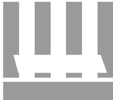
(e) Lateral wet etch using alkaline solution - Smoothes roughened bottom surfaces - Etches silicon fragments
