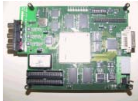
Fig. 5. Hardware board module for conversion graphics(VGA) to DTV with EDAC.
