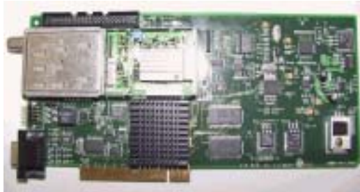
Fig. 8. Hardware Block of DTV receiver module
