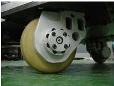
Fig.2. prototype of double-offset active orientable wheel mechanism
