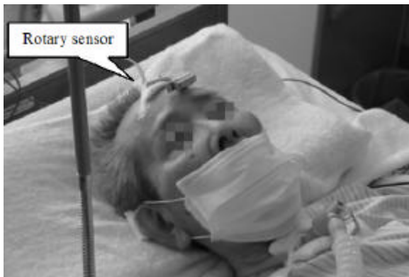
Fig.8. Rotary sensor on eyebrow
