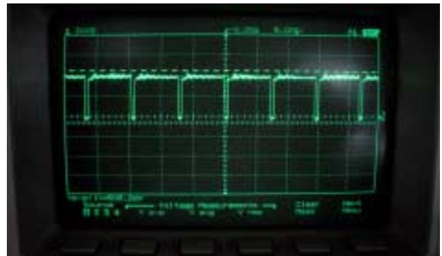
Fig. 8 BRM signal pattern 247, 64 kHz.
