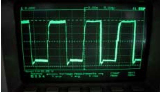
Fig 9 Driven signal of High Frequency Transformer at primary side (64 kHz).
