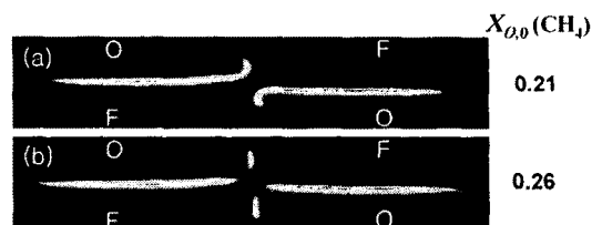
Fig. 8 Direct photographs at \kappa = 20 \text{ s}^{-1} , X_{F,0} = 0.19 ; (a) X_{O,0} = 0.21 , and (b) X_{O,0} = 0.26 .
