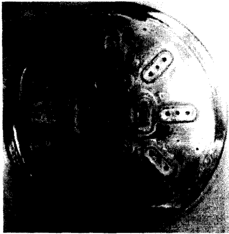
Fig. 2 Injector head of gas generator
