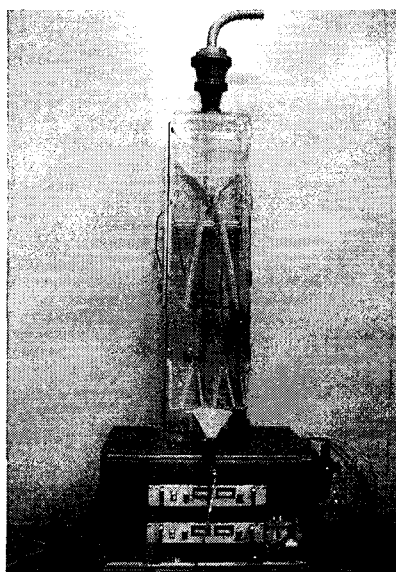
Fig. 1 Principle of Triboelectrostatic Separator developed in this study
