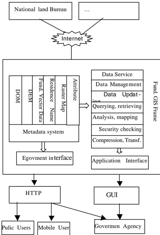
Fig. 1. Structure of FGFDC.
