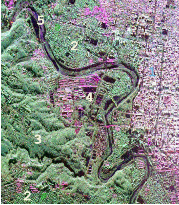
Fig. 1. Pi-SAR L-band FCC image of the test area (1-High density urban, 2-Residential urban, 3-Forest, 4-Ground, 5-Water) (Red=HH, Green=HV, Blue=VV) The size of the area is about 4.1kmx3.5km.
