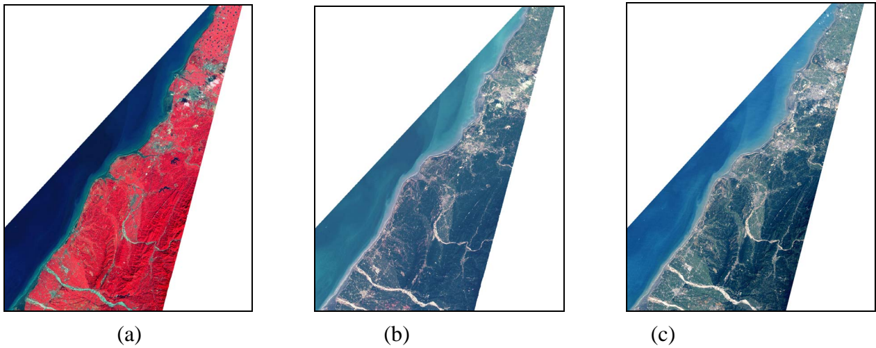
Fig. 2 Images for Test 2: (a) SPOT false color image acquired on 10/31/1995; (b) Simulated true color image generated from (a); (c) Landsat true color image acquired on 10/31/1995.
