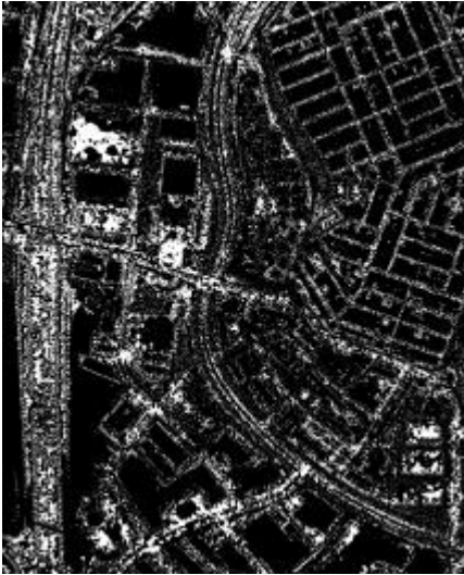
Fig. 4. The object points (black) and ground points (white)
