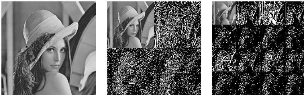
Figure 1. Lenna images and its wavelet decomposition (a) the original Lenna image, (b) two-band wavelet decomposition and (c) four-band wavelet decomposition.
