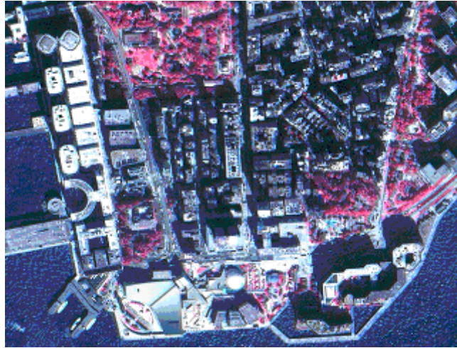
Figure 2. Fused image by four-band wavelet transformation
