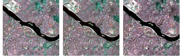
Fig.1. Fused images by using (a) the biorthogonal wavelet transformations, (b) the orthonormal wavelet transformation, and (c) IHS method, respectively.
