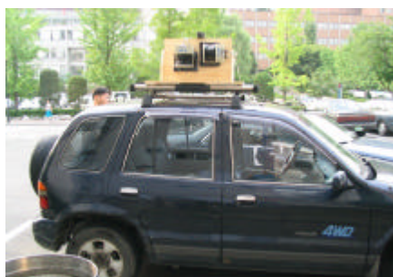
Fig. 1. Data acquisition system
