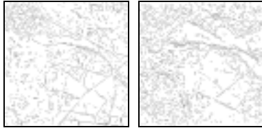
Fig. 5. Feature lines extracted by using Förstner operator in aerial ortho image (left) and TOPSAR image (right) in the test area A.
