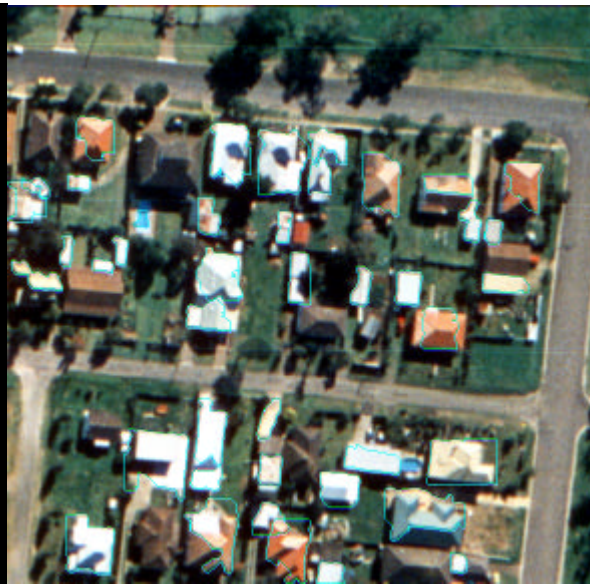
Figure 3 Extracted buildings overlaid on ortho image
