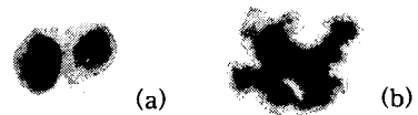
Fig. 1. (a) 2 combined Al 2 O 3 particles coated with ultrafine SiO 2 particles, (b) agglomerated particles
