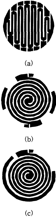
Fig. 1. The pattern shapes of current limiting elements. (a) meander, (b) bi-spiral, (c) spiral shape
