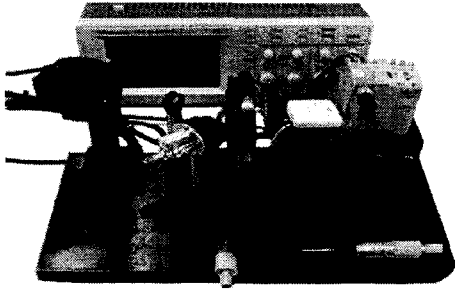
Fig. 3 Burr measurement device using the laser
