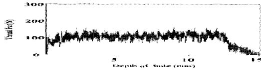
Fig.1 Relation between hole depth and thrust on GFRP for HSS, V=62.4\text{m/min} , f=0.1\text{mm/rev}
