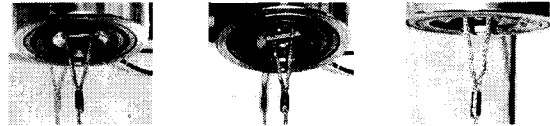
(a) Installation (b) 60kN loading (c) 65kN~fracture Fig. 4-6 Stress concentration at wire rope splice eye
