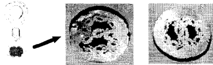
Fig. 4-3 Rope Size 12mm Steel Pipe Cross Section
