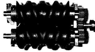
Fig.12 Screw intermeshing equipment
