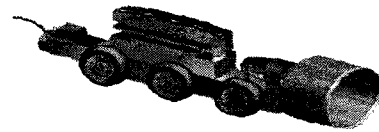
Fig. 9 The whole 3D-modeling of cutting unit of projecting parts connects with interior parts of drainpipe
