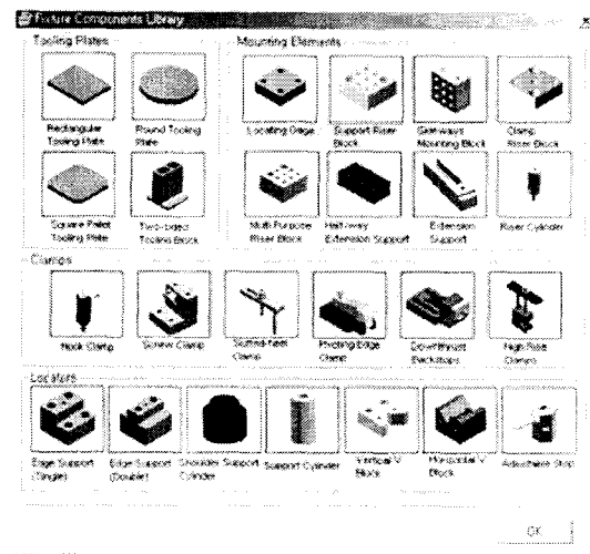
Fig.4 Fixture components library of I-Fix system
