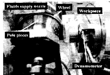
Fig.3 Photograph of the MR polishing process
