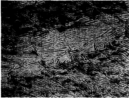
Fig. 5. The microstructure of sample forged at 800°C, 0.001s -1 .
