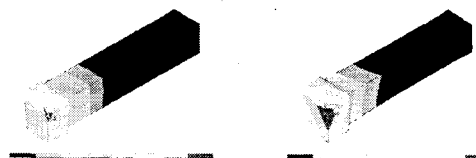
a. temperature distribution b. displacement (USUM) Fig. 2 Temperature and displacement when tool tip temperature is 900℃
