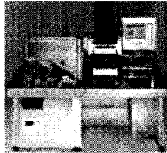
Fig.1 EVG 620 imprinting lithography equipment
