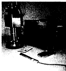
Figure 1. Portable SMPS+C (Fast Sequential Mobility Particle Sizer and Counter) with the medium classifier, a climatic sensor and a mobile phone adapter.
