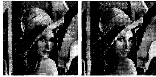
Figure 9: Reconstructed images, hard threshold (left: RMSE = 21.23), soft threshold with condition 3 (right: RMSE = 18.53)
