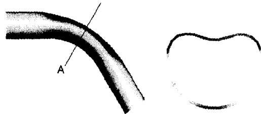
Fig. 2 Thinning distribution after bending simulation without mandrel and the section A
