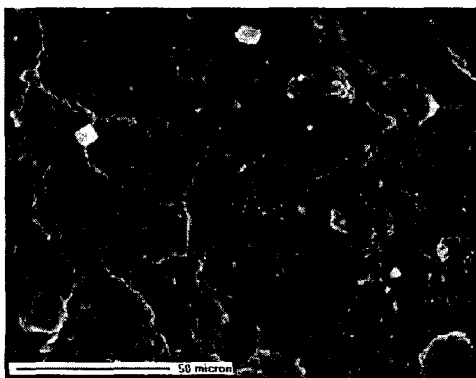
Fig. 1 SEM micrograph of PP compounded with particle size 6micron CaCO 3
