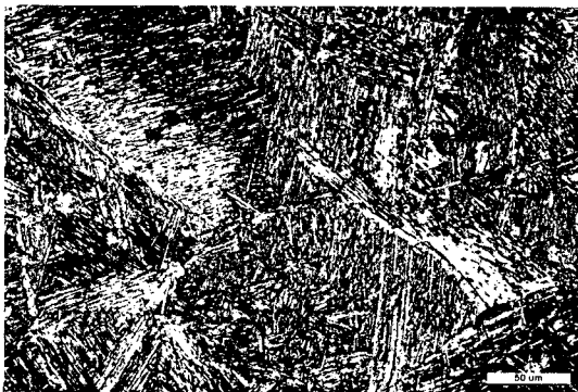
Fig. 1 Microstructure of synthetic HAZ subjected to thermal cycle ( \Delta t_{800-500}=3\text{sec} ).
