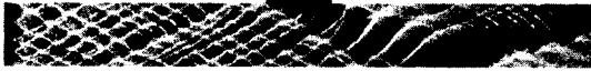
Fig. 2 Numerical smoked-foil record (maximum pressure distribution at each location over an entire computing time) of two-dimensional detonation wave propagating in T-branched flame tube.
