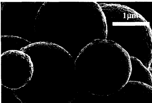
Figure 2. SEM image of Carbonyl Iron particles.
