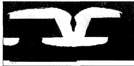
FIGURE 8. The imaging system permits control of beam profile at the target, resulting in uniform microvia holes.
