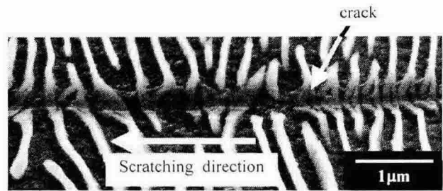
Fig.6 Deformation and fracture of lamellar cementite in groove scratched on pearlite
