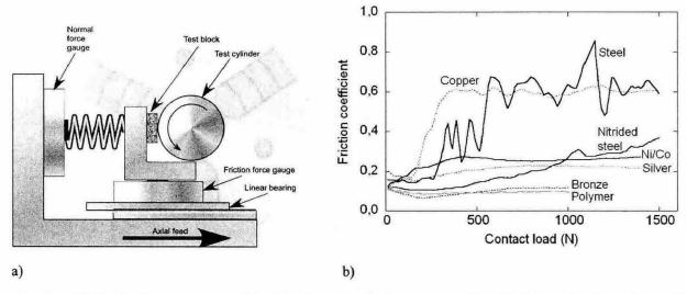
Fig. 1. a) Principal test set up of the block-on-cylinder test used in this investigation. Through the spring loading, it is possible to scan the contact load during each test run.
