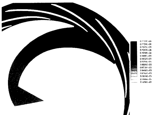
Fig. 4 Pressure distribution in impeller and diffuser of model III for 36520 rpm, 2.39 m³/min
