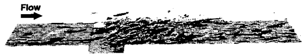
Fig. 8. Iso-surfaces of the streamwise vorticity in case of (d/\theta_b, l/d)=(1.46, 4) at Re=1520 .
