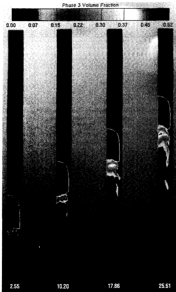
Figure 2. Taylor bubble evolution using the hybrid model. Volume fraction field tracked by the multifluid model (phase 3) is plotted at four non-dimensional times (denoted by the numbers inside the frames). A white solid-line in each frame is an iso-contour of the air volume fraction (phase 2), tracked by the VOF model. The background fluid (phase 1) is water.
